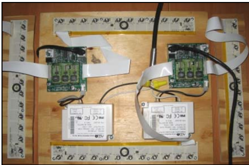
Figure 2 – MCU, Driver, and LEDs
